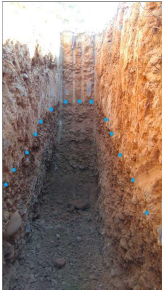
Plate 7-1: The gravelly layer as exposed within a test pit (this view test pit LC22); the boundary indicated by the dotted line
